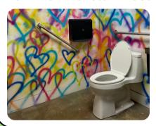
McCabe installed low-flow toilets in their most frequently used bathrooms, reducing water usage from 6L to 4.8L per flush. This change will help lower their water bill and contributes to their goal of reducing overall water usage by 10%
